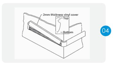
Retain the vinyl cover and trim the interface between the ends of the cover and the elbow with a file
