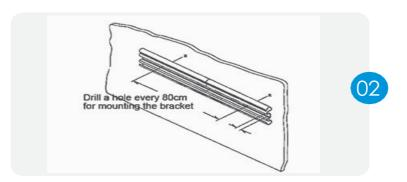
Install elbows on both sides of the aluminumprofile, fix them with screws, and then punch holes in the corresponding positions of the aluminum profiles, and then fix them on the wall
