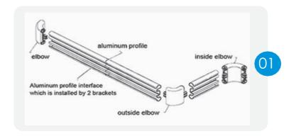
Place a horizontal line on the wall (the bottom of the handrail is 80-85CM from the ground) The bracket is fixed to the wall and the position of the bracket is fixed from the distance of 25cm from the frame of the two sides, and is evenly distributed around 80cm, Measure the actual length between the door frames, and then subtract 16cm(two elbow lengths) from the actual length to cut the aluminum alloy profile
