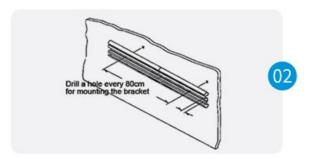
Install elbows on both sides of the aluminum profile, fix them with screws, and then punch holes in the corresponding positions of the aluminum profiles, and then fix them on the wall.
