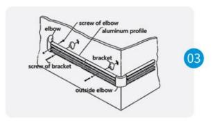
After fixing the aluminum profile, measure the distance cut the between the elbows on both sides, and then cut the vinyl cover. Before the cutting of vinyl cover, the two ends of the material should be trimmed first.
