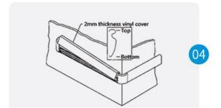
Retain the vinyl cover and trim the interface between the ends of the cover and the elbow with a file.
