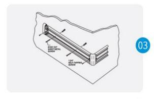
Drill marked holes on wall using a 1/4"drill bit and position Alligator anchors into holes. Mount retainer on wall and tighten screws to secure. Slide end caps and corners onto the retainer and secure. leaving a 1/16" gap between returns/corners and retainer to allow for adjustment. See Figure 3.
