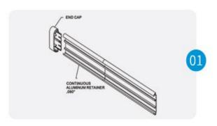
Cut the aluminum retainer to the desired length, leaving allowance for end cap (See figure 1)
