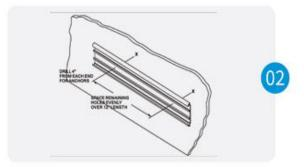
Drill holes in centerline of retainer using 1/4"drill bit. Position retainer on wall allowing for end caps/corners. Level and mark holes. See Figure 2.
