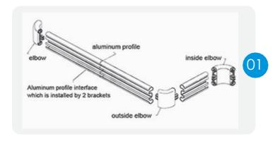
Place a horizontal line on the wall (the bottom of the handrail is 80-85CM from the ground) The bracket is fixed to the wall and the position of the bracket is fixed from the distance of 25cm from the frame of the two sides, and is evenly distributed around 80cm, Measure the actual length between the door frames, and then subtract 16cm(two elbow lengths) from the actual length to cut the aluminum alloy profile
