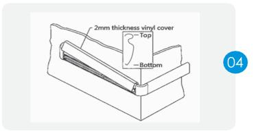
Retain the vinyl cover and trim the interface between the ends of the cover and the elbow with a file
