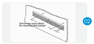
Install elbows on both sides of the aluminumprofile, fix them with screws, and then punch holes in the corresponding positions of the aluminum profiles, and then fix them on the wall
