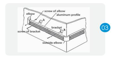
After fixing the aluminum profile, measure the distance between the elbows on both sides and then cut the vinyl cover Before the cutting of the vinyl cover, the two ends of the material should be trimmed first
