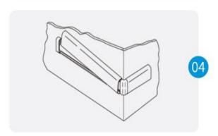
Cut the impact bumper to the length between the inside edge of the end caps/corners. Position and snap bumper in place. Cut the cover to length between end caps and/or corners. (Note: Trim factory edges square before installation). Position cover on retainer and adjust returns and/or corners for a tight fit. Push cover over the retainer until snaps into place. See Figure 4.
