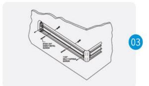
Drill marked holes on wall using a 1/4" drill bit and position Alligator anchors into holes. Mount retainer on wall and tighten screws to secure. Slide end caps and corners onto the retainer and secure, leaving a 1/16" gap between returns/corners and retainer to allow for adjustment. See Figure 3.
