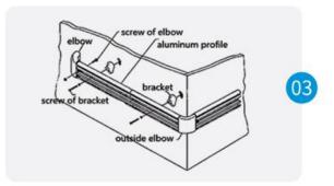
After fixing the aluminum profile, measure the distance cut the between the elbows on both sides, and then cut the vinyl cover. Before the cutting of vinyl cover, the two ends of the material should be trimmed first.
