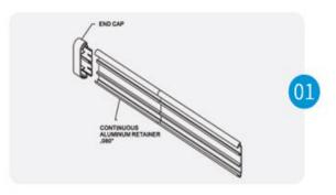
Cut aluminum retainer to desired length, leaving allowance for end caps, See Figure 1.
