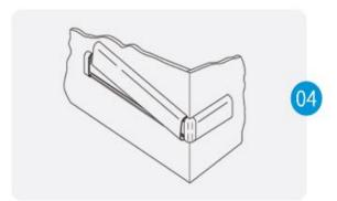
Cut the impact bumper to the length between the inside edge of the end caps/corners. Position and snap bumper in place. Cut the cover to length between end caps and/or corners. (Note: Trim factory edges square before installation). Position cover on retainer and adjust returns and/or corners for a tight fit. Push cover over the retainer untilit snaps into place. See Figure 4.
