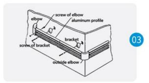
After fixing the aluminum profile, measure the distance between the elbows on both sides, and then cut the vinyl cover. Before the cutting of the vinyl cover, the two ends of the material should be trimmed first. vinyl cover, the two ends of the material should be trimmed first.
