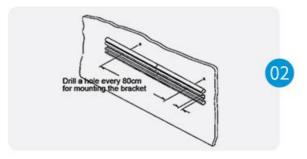
Install elbows on both sides of the aluminum profile, fix them with screws, and then punch holes in the corresponding positions of the aluminum profiles, and then fix them on the wall.
