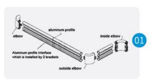
Place a horizontal line on the wall (the bottom of the handrail is 80-85CM from the ground). The bracket is fixed to the wall. and the position of the bracket is fixed from the distance of 25cm from the frame of the two sides, and is evenly distributed around 80cm, Measure the actual length between the door frames, and then subtract 16cm (two elbow lengths) from the actual length to cut the aluminum alloy profile.
