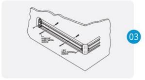
Drill marked holes on wall using a 1/4"drill bit and position Alligator anchors into holes. Mount retainer on wall and tighten screws to secure. Slide end caps and corners onto the retainer and secure. leaving a 1/16" gap between returns/corners and retainer to allow for adjustment. See Figure 3.
