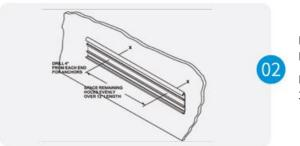
Drill holes in centerline of retainer using 1/4"drill bit. Position retainer on wall allowing for end caps/ DR corners. Level and mark holes. See Figure 2.
