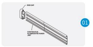
Cut aluminum retainer to desired length, leaving allowance for end caps, See Figure 1.
