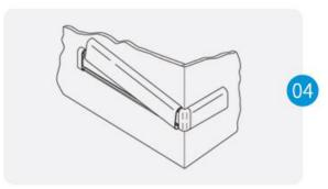
Cut the impact bumper to the length between the inside edge of the end caps/corners. Position and snap bumper in place. Cut the cover to length between end caps and/or corners. (Note: Trim factory edges square before installation). Position cover on retainer and adjust returns and/or corners for a tight fit. Push cover over the retainer untilit snaps into place. See Figure 4.
