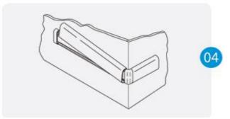
Cut the impact bumper to the length between the inside edge of the end caps/corners. Position and snap bumper in place. Cut the cover to length between end caps and/or corners. (Note: Trim factory edges square before installation). Position cover on retainer and adjust returns and/or corners for a tight fit. Push cover over the retainer untilit snaps into place. See Figure 4.
