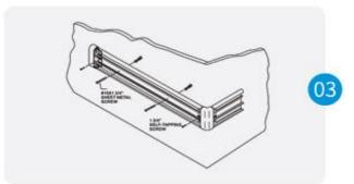
Drill marked holes on wall using a 1/4"drill bit and position Alligator anchors into holes. Mount retainer on wall and tighten screws to secure. Slide end caps and corners onto the retainer and secure. leaving a 1/16" gap between returns/corners and retainer to allow for adjustment. See Figure 3.
