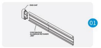
Cut aluminum retainer to desired length, leaving allowance for end caps, See Figure 1.
