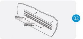
Drill holes in center line of retainer using 1/4"drill bit. Position retainer on wall allowing for end caps/ DR corners. Level and mark holes. See Figure 2.
