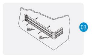
Drill marked holes on wall using a 1/4" drill bit and position Alligator anchors into holes. Mount retainer on wall and tighten screws to secure. Slide end caps and corners onto the retainer and secure, leaving a 1/16" gap between returns/corners and retainer to allow for adjustment. See Figure 3.
