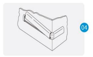
Cut the impact bumper to the length between the inside edge of the end caps/corners. Position and snap bumper in place. Cut the cover to length between end caps and/or corners. (Note: Trim factory edges square before installation). Position cover on retainer and adjust returns and/or corners for a tight fit. Push cover over the retainer until snaps into place. See Figure 4.
